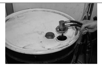
Install fuel pickup fuel hoses to the appropriate couplings at the furnace.
