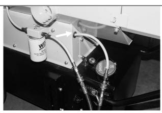
To restore the Dragon for onboard tank use, uncouple the fuel pickup from the Dragon and attach the fuel hoses to the appropriate fittings on the tank as shown.
