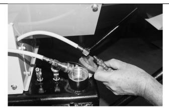
To install fuel pickup on external fuel tank, remove tank cap and insert fuel pickup tube.
