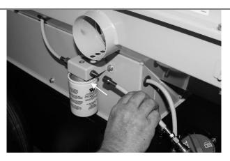
Remove the two fuel hose fittings from tank. Discard fittings.
