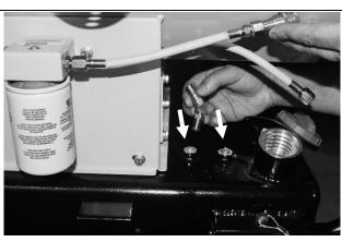
Use 7/16 in. and 9/16 in. wrenches to install the female coupling (B) to the fuel return hose. Do not overtighten.
