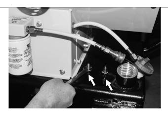
Ensure fittings are properly threaded before tightening. Install fuel intake side/female coupling (C) assembly first, then install the fuel return side/male coupling assembly (D).
