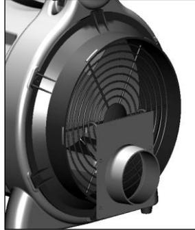
Fasten the black end of the WolfPack Drying System boot to the AirWolf. Use the strap provided to securely fasten and minimize air leaks. Attach the clamp end to the first Vent in line. Check for any air leaks, and install gaskets where needed.
