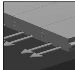
Place WolfPack Drying System Vents in-line and firmly into position. Place Vents up to 10 inches apart, with a piece of L-channel between the Vents. A combination of one to three Vents will cover a linear area between 24 and 118 inches. Be sure each Vent is in the correct position with the air opening facing down. Use as many of the Vents as needed to sufficiently dry the floor.
